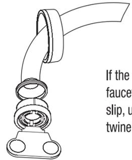
If the front end of the faucet or threaded joint slip, use the sealing tap twine it and tightened
