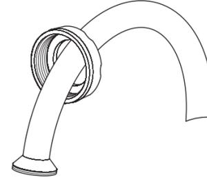
4 Select the appropriate inner threaded connector for installation
