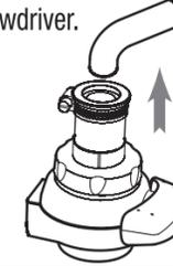
6 If the faucet diameter is 19-24mm, please remove the seal on the universal joint and install it by referring to the installation method.
