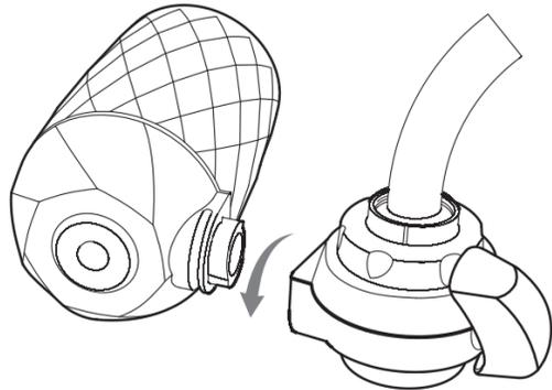
5 Insert the filter base connector into the main unit and tighten it vertically.
