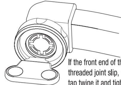
If the front end of the faucet or threaded joint slip, use the sealing tap twine it and tightened
