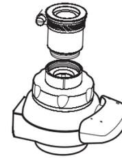
5 Please insert the round faucet into the universal fitting and tighten the retaining ring on the universal joint with a screwdriver.
