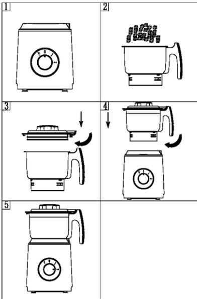
1. Place the main unit on a flat, dry workbench, make sure that the switch knob is set to "0" before turning on the power (see Figure 1), and plug in a power source that meets the requirements on the main unit's nameplate.
