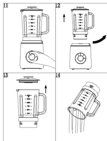
1. Add the right amount of warm water and a small amount of food detergent when cleaning the mixing cup, cover the cup cover and turn the switch knob "P" to run for about 10 seconds (see Figure 11); you can also immerse the mixing cup in water Brush cleaning.
